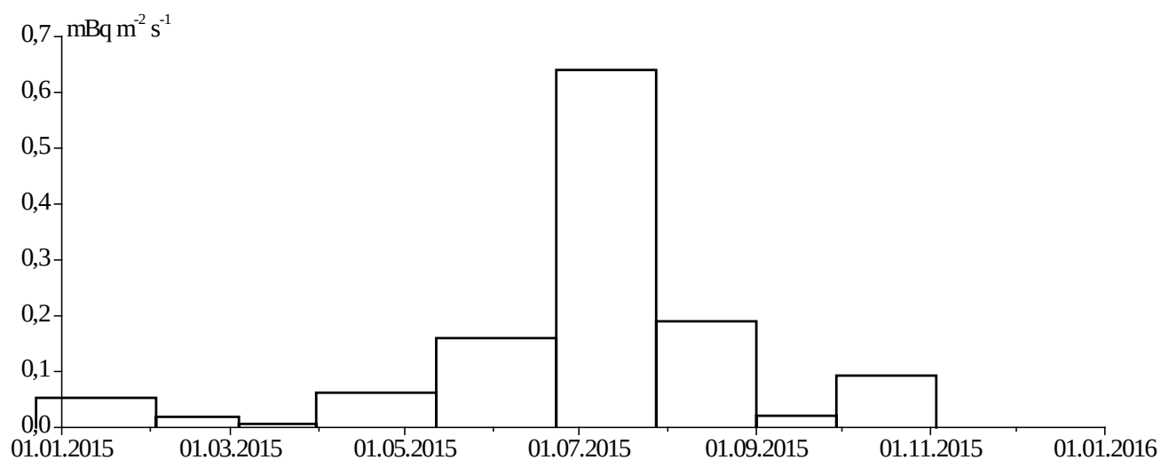
Fig. 3.4 Deposition density of ^{137}\text{Cs} ( in \text{mBq m}^{-2} \text{s}^{-1} ) near the south wall of the machine hall of the "Shelter" with time.
