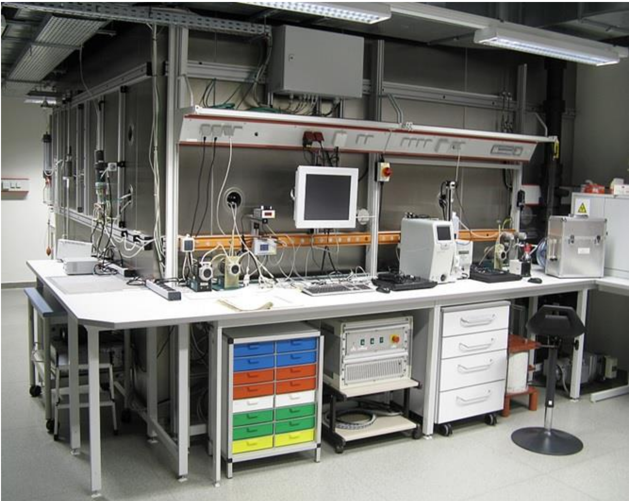
Abbildung 3-1 Kalibrierkammer im Radon-Kalibrierlaboratorium des BfS (Volumen: 30 m 3 ) / Figure 3-1 Calibration chamber in the Radon Calibration Laboratory of the BfS (volume: 30 m 3 )
