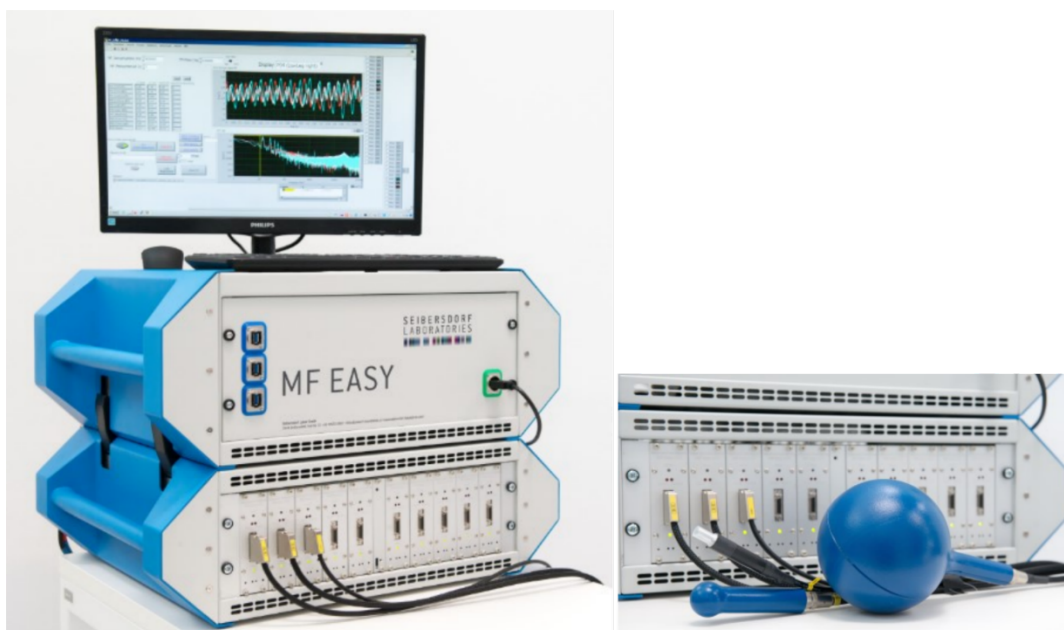
Abbildung 8.1: Verwendetes Magnetfeld-Messsystem MF EASY ( https://rf.seibersdorf-laboratories.at/products-services/products/mf-easy ).
