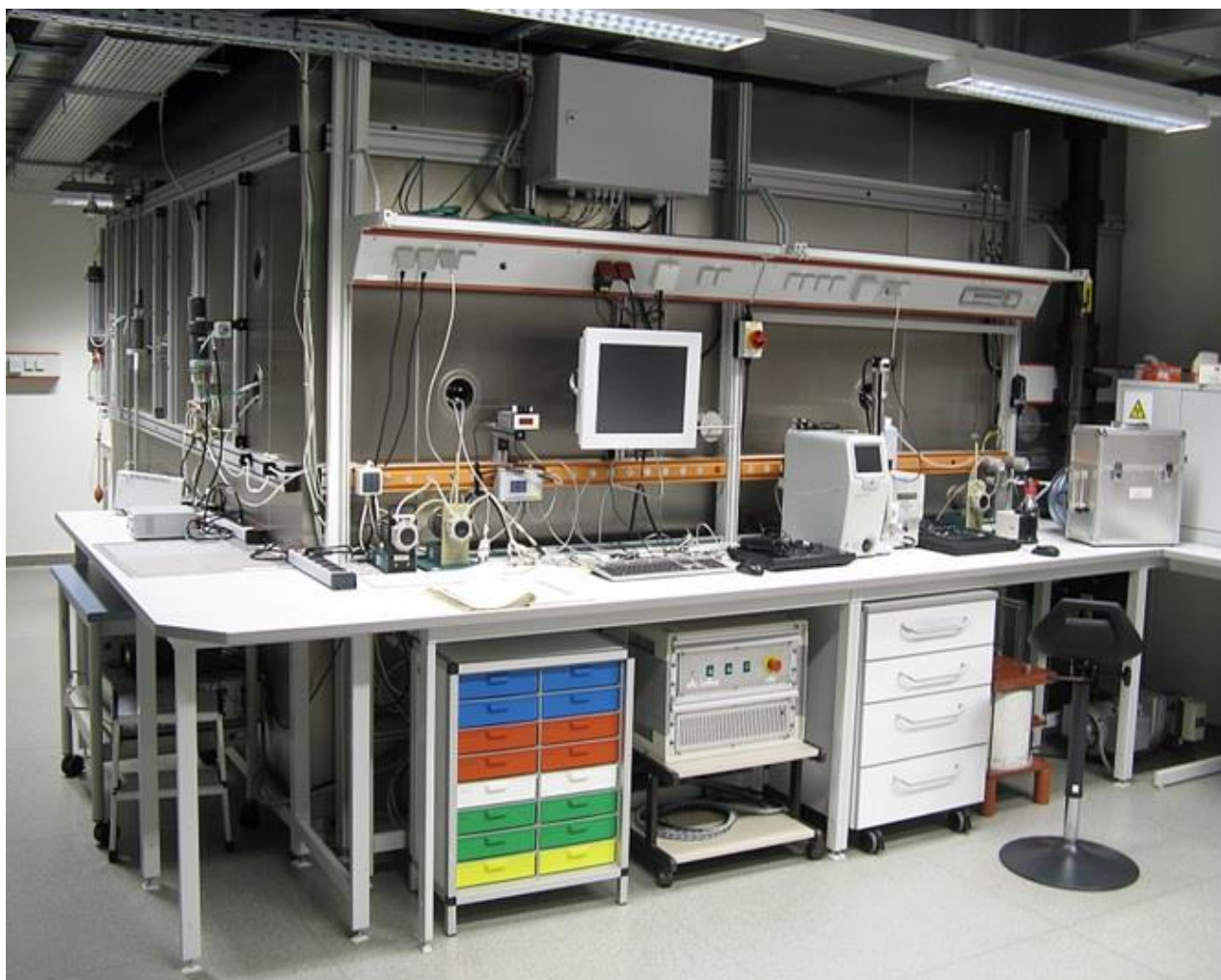
Abbildung 3-1 Kalibrierkammer im Radon-Kalibrierlaboratorium des BfS (Volumen: 30 m 3 ) / Figure 3-1 Calibration chamber in the Radon Calibration Laboratory of the BfS (volume: 30 m 3 )
